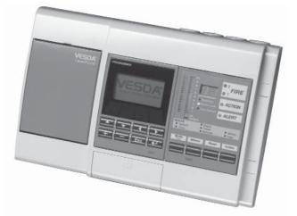
The VESDA VLP detector is the central element of the VESDA ASD product range. Using unique detection principles, the VLP has an alarm sensitivity range of 0.005%–20% obscuration/m (0.0015%–6.25% obscuration/ft). The VLP is classed as a "Very Early Warning Smoke Detector", which means that it detects fire at the earliest possible stage and reliably measures very low to extremely high concentrations of smoke.
