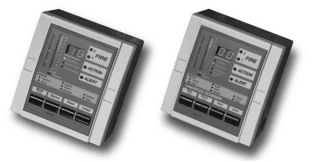
Display modules provide real-time indication of the status of a VESDA detector. They have a 20-segment vertical bar graph display, a 2 digit numeric display, an audible sounder, clear alarm and fault indicators. They also have 4 push button keys to control the detector and the mode of the display.
