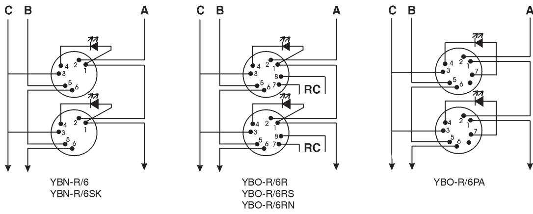
**RC** Relay Contacts - a flying lead on either terminal 7 or 8 selects either N/C or N/O (supplied as N/C)
